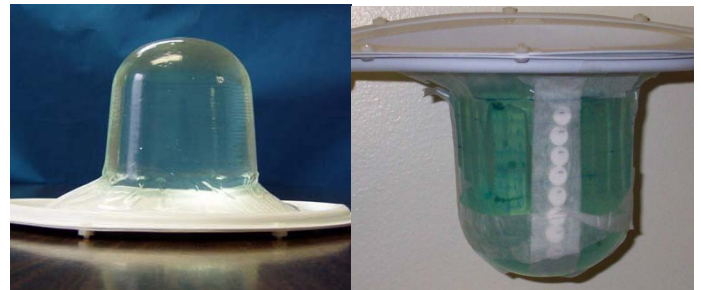
Fig. 1. Deformable breast phantom. Left : supported on its base. Right : suspended in orientation used in experiments. The diameter (neglecting the base) is approximately 10 cm. See text for details.
